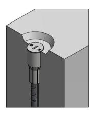
After removing the KU nailing plate, mount the plastic plug inside the socket.
